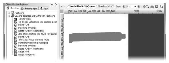
Insert a new check function **Determine Threshold** and a new check function **Create ROIs by Thresholding** before the comment check function 2nd step: ....
