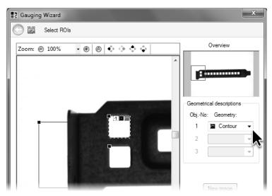
Select the ROI describing the upper hole and select **Contour** as geometry to gauge the hole's width.
