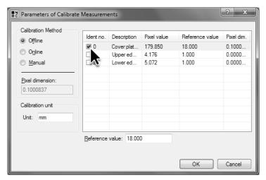
3 In **Offline** mode, the calibration factor is calculated from the selected measurements upon closing the parameter dialog.
