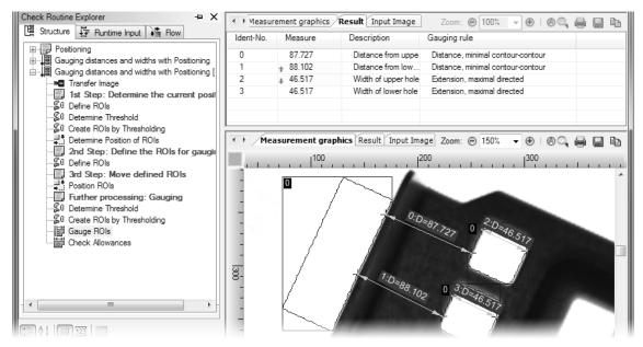
With the traced angle, the width of the holes is gauged.
