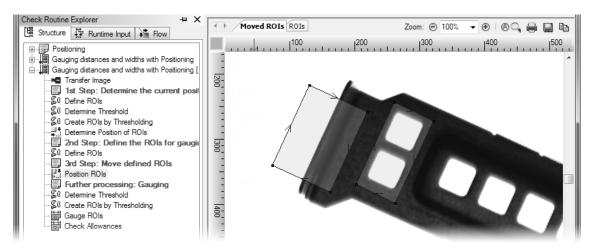
**5** The position of the ROIs is also compensated for rotated objects.
