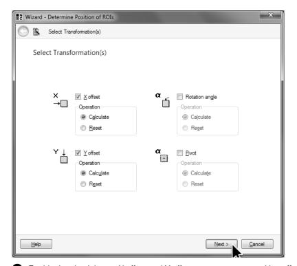
**9** Enable the check boxes X offset and Y offset to compensate position offsets.
