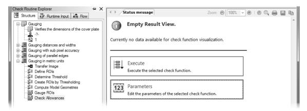
1 Select the check function **Check Allowances** to insert a new check function before it.
