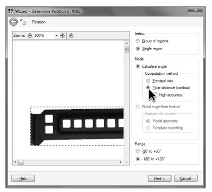
2 The option Polar distance (Contour) offers a more precise determination of the Rotation angle.
