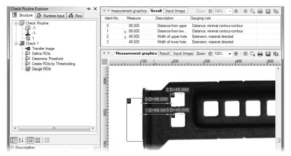
The **Result** tab displays the results and gauging rules in a table. The **Measurement graphics** tab of the result view displays the measurements graphically in the image.
