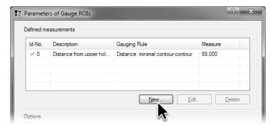
3 Click the **New...** button to define another measurement for gauging the distance between the bottom hole and the edge.
