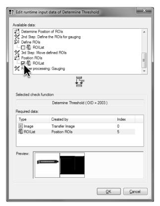
The input data assignment of the two imported check functions **Determine Threshold** and **Determine ROIs by Thresholding** must be changed so the ROIs are used whose position were changed.
