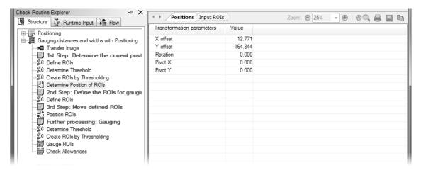
The check function **Determine Position of ROIs** measures the offset of the cover plate's position in the image.
