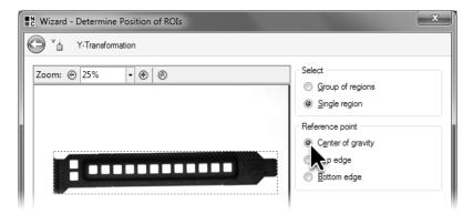
Select **Center of gravity** as reference point for determining the offset in the Y direction.
