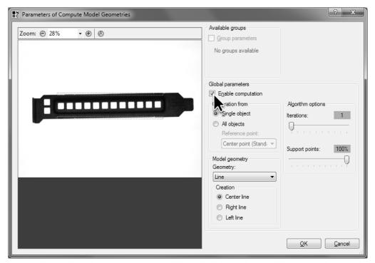
Activate computation of model geometries to replace the created contours with lines.
