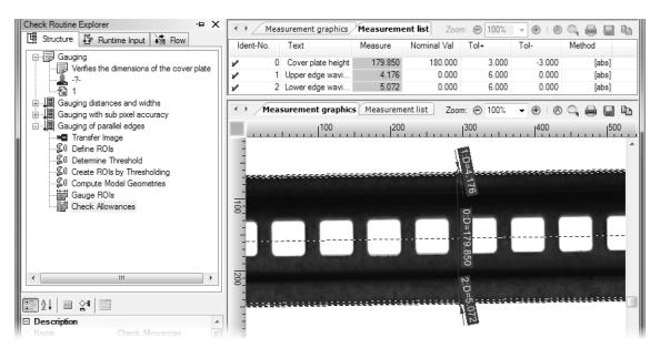
15 The measurements are displayed in the result view together with the auxiliary lines necessary for gauging.
