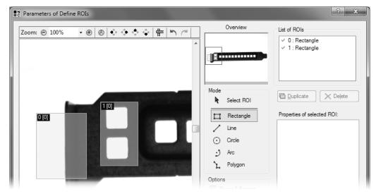
1 In the parameter dialog of **Define ROIs** define an ROI on the left edge of the cover plate and a second ROI over the two left holes.
