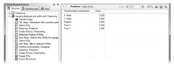
For the image we used to teach the reference values, the offset for the reference values is zero.
