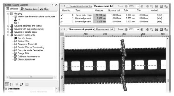
After calibrating the measurements, the target values and allowances can be entered using metric values in **Check Allowances**.
