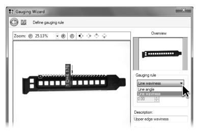
Select the gauging rule **Line waviness** to check the upper edge of the cover plate for indentations.
