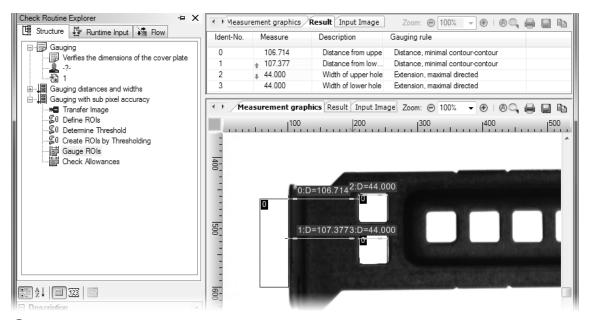
4 Because of sub-pixel computation the distances of the holes from the edge are gauged with sub-pixel precision.
