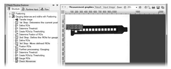
After position adjustment, the width and the distance between the holes can be measured.
