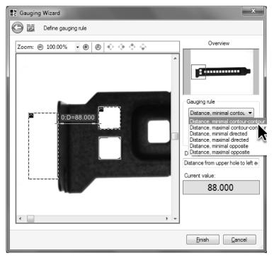
For the Gauging rule select Distance, minimal contour-contour to gauge the distance between edge and hole.
