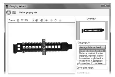
Select the gauging rule **Average distance**, **line-line** to gauge the height of the cover plate.
