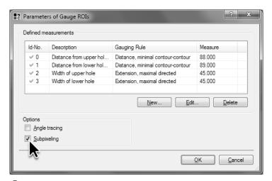
3 Enable the **Subpixeling**, option to compute more precise and threshold-independent gauging results.
