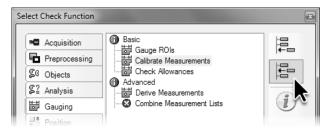
2 Insert the check function Calibrate Measurements into the check.
