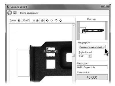
As gauging rule select Extension, maximal directed and keep Angle direction at 0°.
