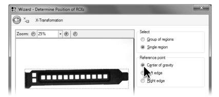
Select Center of gravity as reference point for determining the offset in the X direction.
