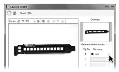
Select the ROI on the upper edge of the cover plate and select **Line** geometry.
