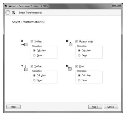
1 To compensate the object's rotation, the **Rotation angle** and the **Pivot** must be determined during teaching.
