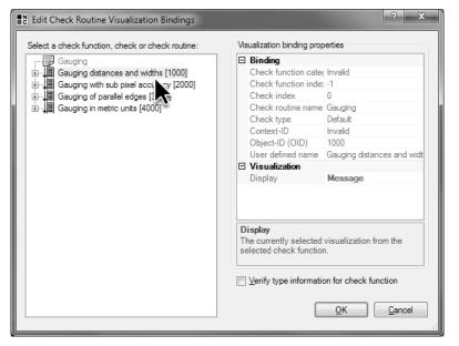
6 Select the check Gauging distances and widths to display its results.
