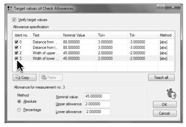
In the target value dialog of the check function **Check Allowances** the target values and the upper and lower allowances are configured for every measurement.
