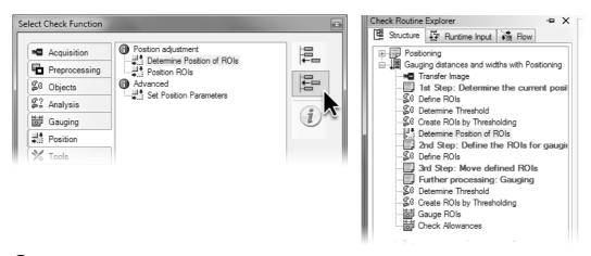
8 Insert a new check function **Determine Position of ROIs** before the comment check function *2nd step:* ....
