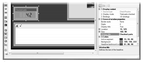
Draw a window of the **Counter** type in the screen layout to display the number of pieces inspected.
