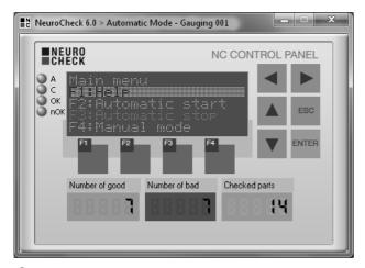
2 In automatic mode, the selected Control Panel is used. When changing the Control Panel the menu remains unchanged.
