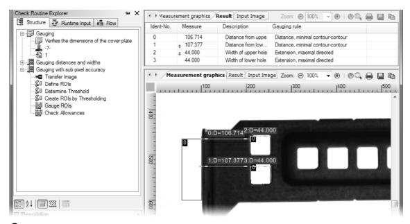
Because of sub-pixel computation the distances of the holes from the edge are gauged with sub-pixel precision.
