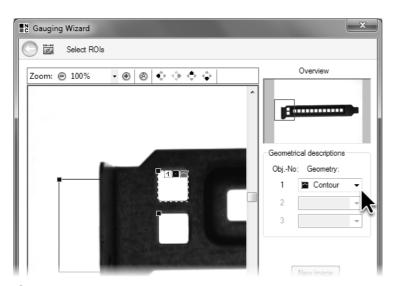
**(1)** Select the ROI describing the upper hole and select **Contour** as geometry to gauge the hole's width.
