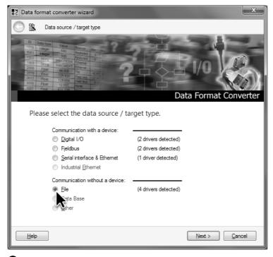
2 In the Data Format Converter Wizard select File to integrate a file converter.
