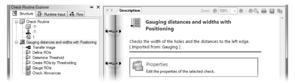
3 Delete the automatically created empty check and change the name of the imported check.
