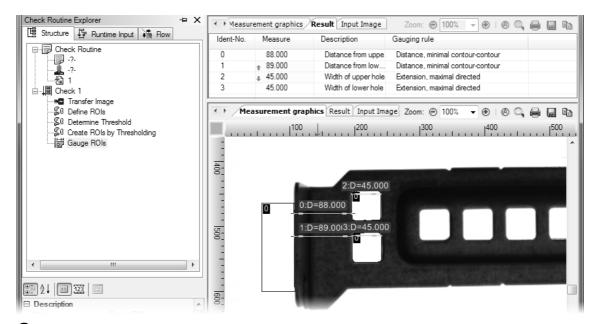
The Result tab displays the results and gauging rules in a table. The Measurement graphics tab of the result view displays the measurements graphically in the image.
