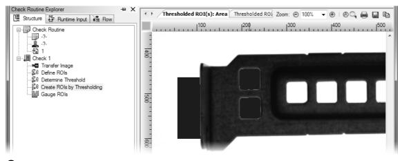
3 The background on the left edge of the cover plate is bordered on three sides by the search area and only on the right side by the object edge.
