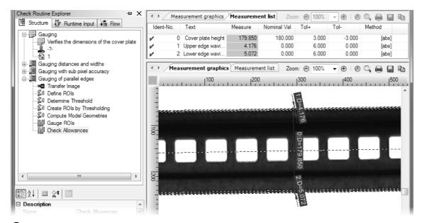
The measurements are displayed in the result view together with the auxiliary lines necessary for gauging.
