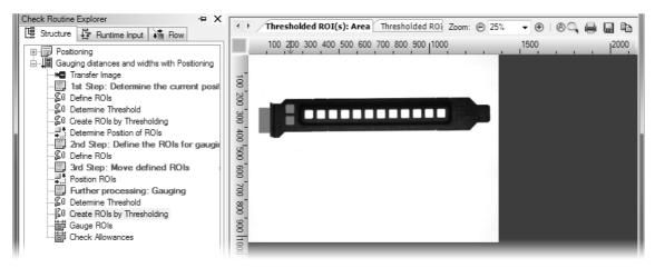
After position adjustment both the background and the holes are found even if the cover plate position has changed.
