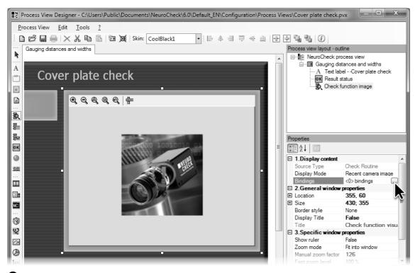
Draw a window of the Check function image type in screen layout.
