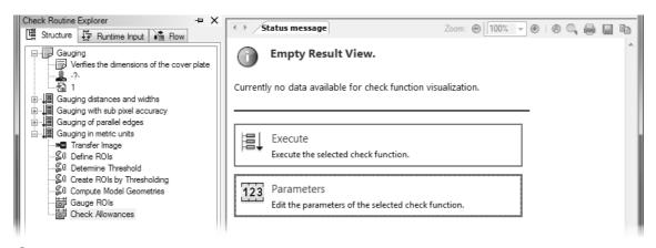
1 Select the check function Check Allowances to insert a new check function before it.
