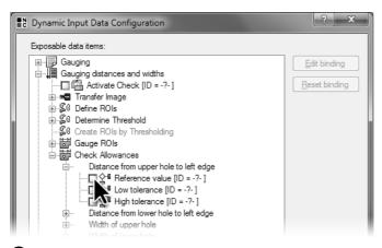
From the Check routine menu select Data Input and in the Dynamic Input Data Configuration dialog select the target value you want to change in automatic mode.
