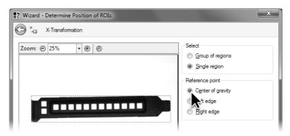
Select Center of gravity as reference point for determining the offset in the X direction.
