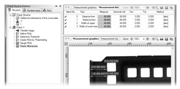
In the Measurement graphics tab of the result view, measurements within the configured allowances are highlighted in green. In the Measurement list tab, these measurements are highlighted in green.
