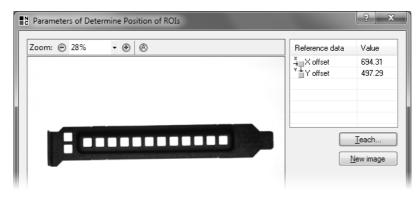
Description: The parameter dialog displays the reference values for the offset compensation.
