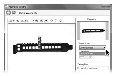
Delect the gauging rule Line waviness to check the upper edge of the cover plate for indentations.
