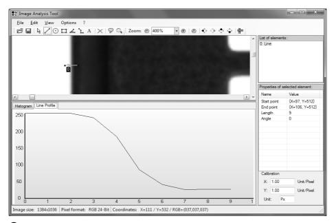
2 The transition between cover plate and background is distributed over several camera pixels, which is used for determining the position of the edge with sub-pixel precision.
