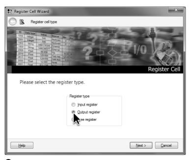
On the first page of the **Register Cell Wizard** select the **Output register** option for the new register cell.
