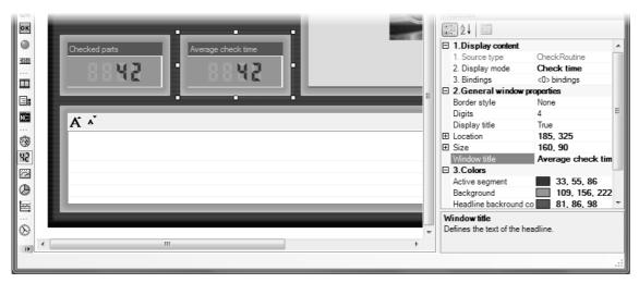
Draw another window of the Counter type in the screen layout to display the average execution time of the check.
