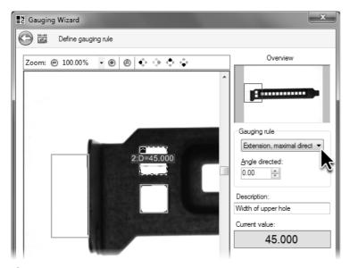
As gauging rule select Extension, maximal directed and keep Angle direction at 0°.
