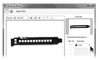
**①** Select the ROI on the upper edge of the cover plate and select Line geometry.
