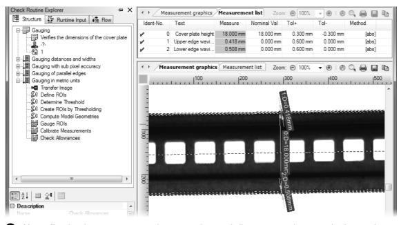
6 After calibrating the measurements, the target values and allowances can be entered using metric values in Check Allowances.
