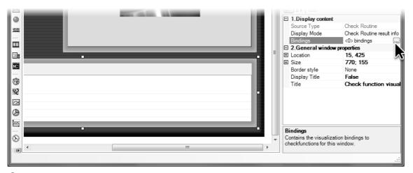
Oraw a window of the Check function visualization list type in the screen layout to visualize the gauging results.
