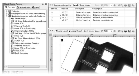
8 With the traced angle, the width of the holes is gauged.
