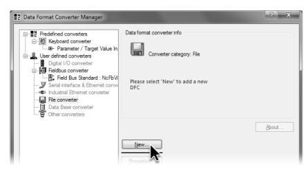
1 Click New... in the Data Format Converter Manager to integrate a new converter.
