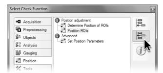
Insert the check function **Position ROIs** to adjust the position of the ROIs.
