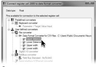
In the Connect register cell 2000 to data format converter dialog, select the pin you want to use for the output of the register cell values.
