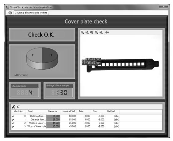
(L) In automatic mode, the check routine results are displayed in the process view.
