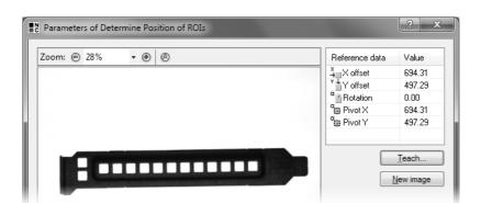
4 The parameter dialog displays the reference values for the offsets, the angle and the pivot.
