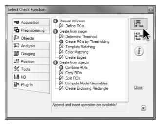
6 Add the check function **Compute Model Geometries** to the check.
