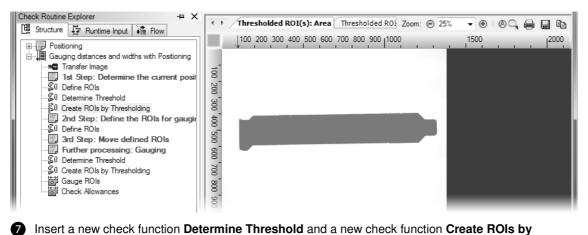
Insert a new check function **Determine Threshold** and a new check function **Create ROIs by Thresholding** before the comment check function *2nd step:* ....
