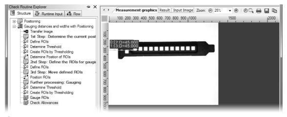
22 After position adjustment, the width and the distance between the holes can be measured.
