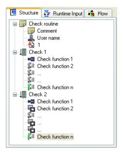
A **check routine** typically consists of several individual checks (or simply: **checks**) inspecting different aspects of the work piece.
