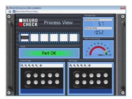
In a real-world production line inspection system, check routine execution in automatic mode will typically be started by an external signal from a PLC or master computer. The signal will for instance be transferred via digital inputs or Ethernet. General configuration options for external control and communication are set by choosing **Remote Control** from the **System** menu in Manual Mode.
